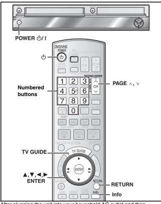
After plugging the unit into your household AC outlet and then pressing [ $\circlearrowleft$ , DVD/VHS POWER] to turn the unit on for the first time, the unit starts language, TV aspect type and TV Guide On Screen® system setup.
